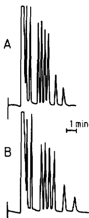
Fig. 3. Demonstration of flow compensation. Separation of C_{10} - C_{22} n -alkanes. Column, 250\text{ mm} \times 4.1\text{ mm} I.D., packed with RP-18, 10\text{ }\mu\text{m} . Pressure programme, 92-184 bar, linear in 2.5 min. Temperature, 40^\circ\text{C} . A, With flow compensation; B, without flow compensation.
